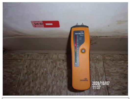
Photo #25 - Moisture meter at red level reading, Unit #1260 living room
