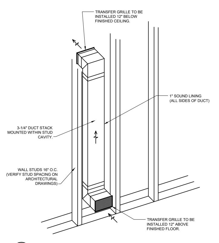
8 RETURN AIR TRANSFER DUCT STACK IN STUD WALL
