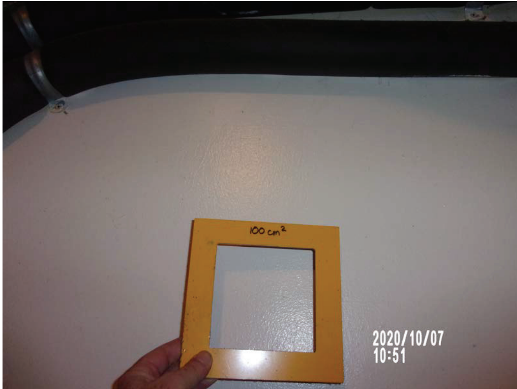
Photo #7 – Swab sample #70-02, Unit #1270 laundry room
