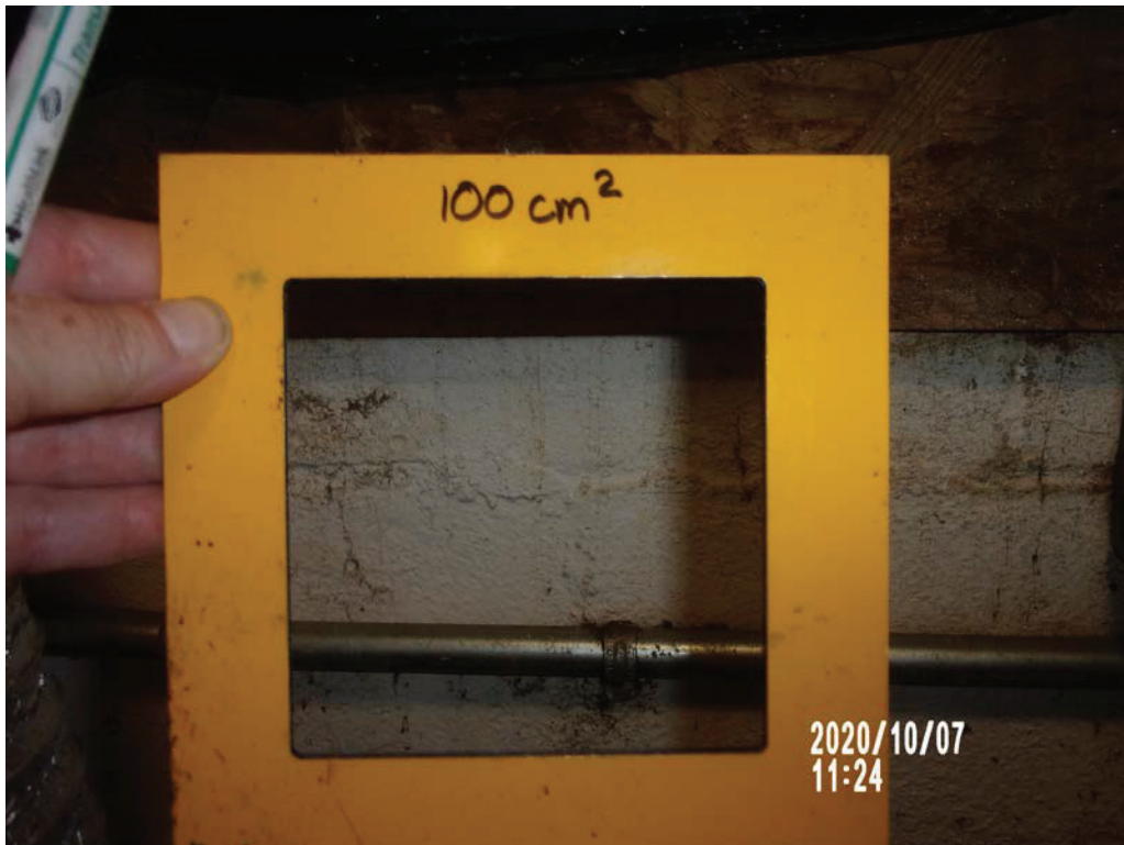
Photo #20 – Swab sample #64-02, Unit #1264 laundry room
