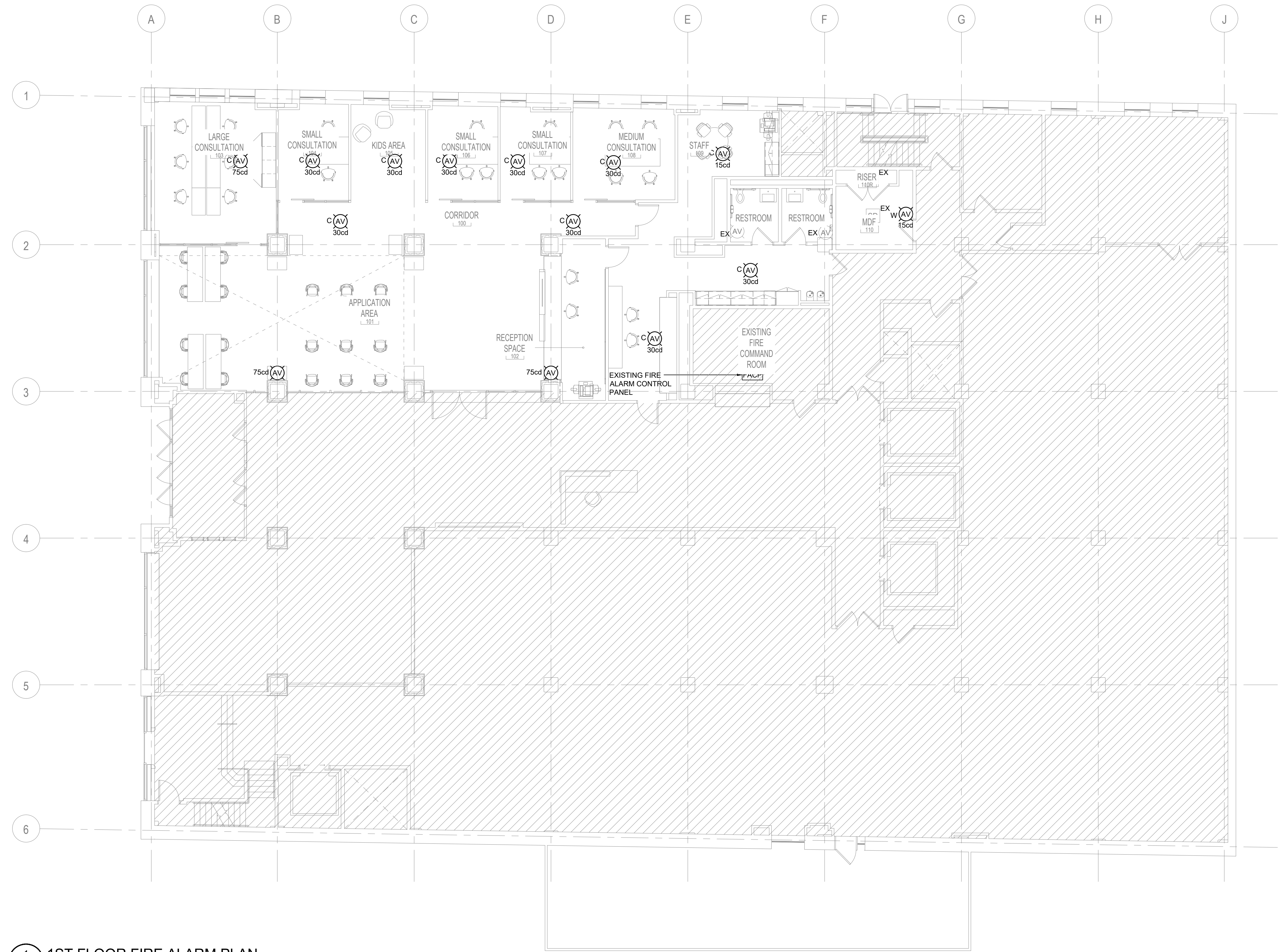
1 1ST FLOOR FIRE ALARM PLAN E-401 1/8" = 1'-0"
